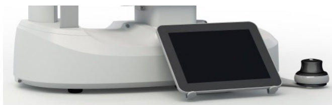
Fig. 11 – EIDON Custom Control Interface and 3D Joystick mounted on the left side of the device
