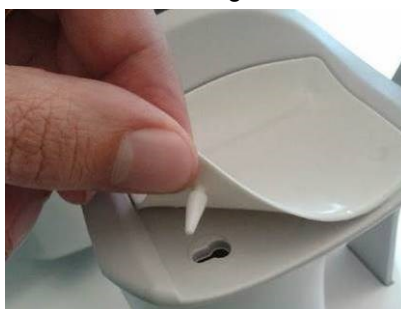
Fig. 103 – Removal of the chin rest silicone pad
