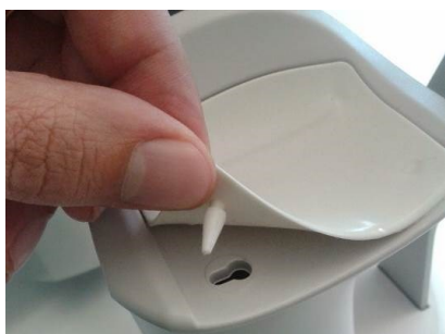
Fig. 191 - Removal of the chin rest silicone pad
