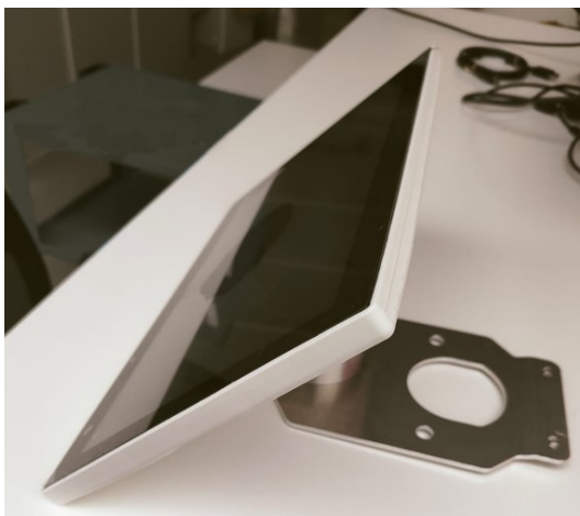
Fig. 8 – The embedded display fixed to its support bracket plate
