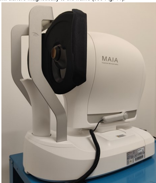
Fig. 11 – Magnetic Light Shield mounted on MAIA
